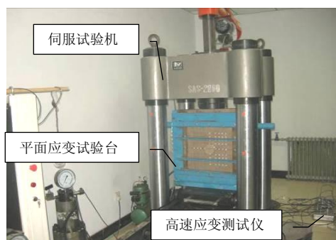
图 4 CM60/10 试验台加载 Fig.4 CM60/10 test-bed loading
