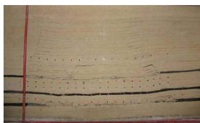
图 4 3-2 煤 N3 面开采后上覆岩层形态 Fig.4 Overburden rock stratum after N3 panel, 3-2 coal seam mined
