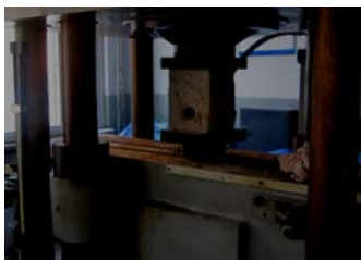
图 9 试样加压 Fig.9 Pressed sample
