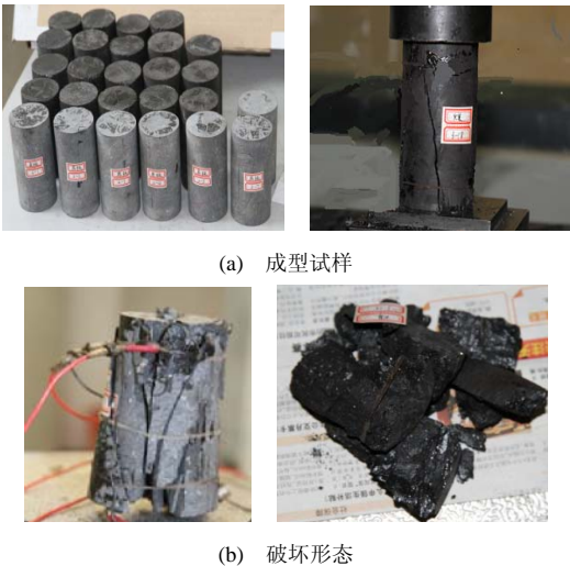
图 4 煤、岩试样试验前后形态图 Fig.4 The shapes of coal and rock in experiment
