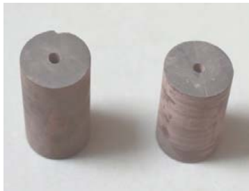
图 8 实验用的泥岩试件(钻孔 \Phi 10\text{ mm} ) Fig.8 The samples(borehole \Phi 10\text{ mm} )
