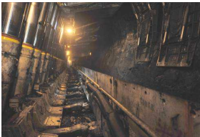
图 1 7.0 m 支架综采面井下照片 Fig.1 Underground photograph of the fully mechanized face with 7.0 m support
